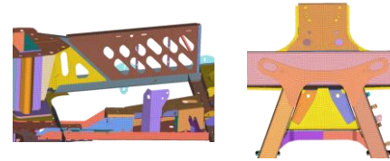
Sheet Metal Mesh with properties
